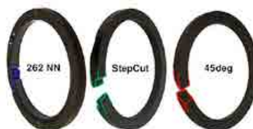
Figure 6: Piston rings tested: 45deg inclined cut, step cut, 262 NN.
